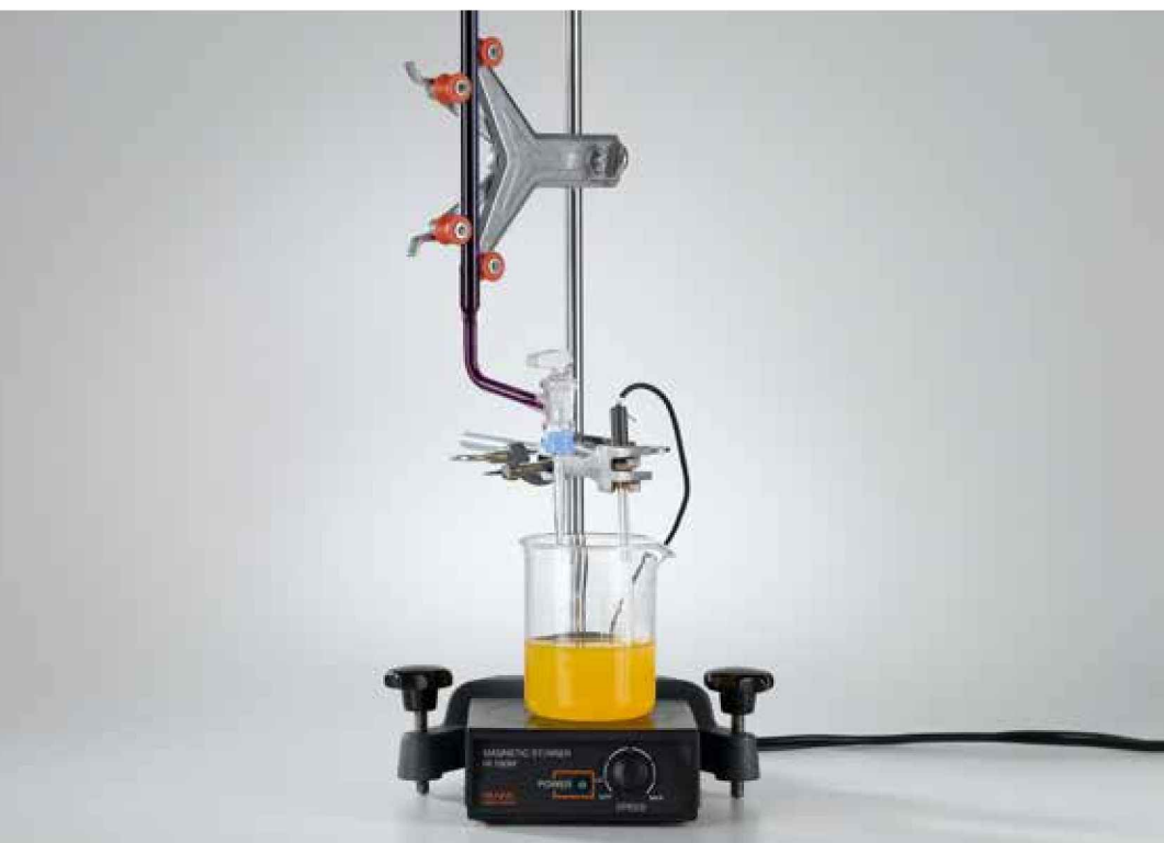
Manganometric determination of iron(II) ions (C3.5.3.2)
